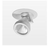
Semi-recessed luminaire with LED, rated life of the LED L80/B10 > 50000 h, colour rendering index CRI > 90, chromaticity tolerance 2 SDCM (initial), reflector with circular light distribution pattern, reflector pure aluminium 99,99% in MIRO-Silver®, segmented and faceted, 3D lens silicon to reduce the proportion of scattered light, die-cast aluminium, powder-coated, rotation angle 400°, swivel angle +85° / -85°, stratowhite, separate driver unit
