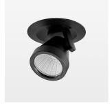
Semi-recessed luminaire with LED, rated life of the LED L80/B10 > 50000 h, colour rendering index CRI > 96, chromaticity tolerance 2 SDCM (initial), reflector with circular light distribution pattern, reflector pure aluminium 99,99% in MIRO-Silver®, segmented and faceted, 3D lens silicon to reduce the proportion of scattered light, die-cast aluminium, powder-coated, rotation angle 400°, swivel angle +85°/-85°, stratoblack, potentiometer to adjust the brightness, separate driver unit
