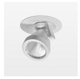
Semi-recessed luminaire with LED, rated life of the LED L80/B10 > 50000 h, colour rendering index CRI > 96, chromaticity tolerance 2 SDCM (initial), reflector with circular light distribution pattern, reflector pure aluminium 99,99% in MIRO-Silver®, segmented and faceted, 3D lens silicon to reduce the proportion of scattered light, die-cast aluminium, powder-coated, rotation angle 400°, swivel angle +85°/-85°, stratowhite, potentiometer to adjust the brightness, separate driver unit
