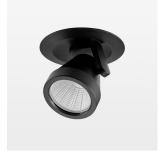
Semi-recessed luminaire with LED, rated life of the LED L80/B10 > 50000 h, colour rendering index CRI > 96, chromaticity tolerance 2 SDCM (initial), reflector with circular light distribution pattern, reflector pure aluminium 99,99% in MIRO-Silver®, segmented and faceted, die-cast aluminium, powder-coated, rotation angle 400°, swivel angle +85°/-85°, stratoblack, potentiometer to adjust the brightness, separate driver unit
