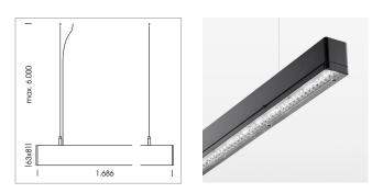
Light band with LED, rated life of the LED L80/B50 > 50000 h, colour rendering index CRI > 80, reflector with homogeneous light distribution pattern, lens optics made of PMMA, luminaire insert sheet steel, powder-coated, black
