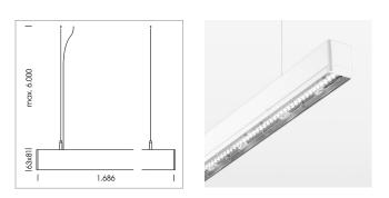
Light band with LED, rated life of the LED L80/B50 > 50000 h, colour rendering index CRI > 80, reflector with double asymmetrical light distribution pattern, lens optics made of PMMA, luminaire insert sheet steel, powder-coated, white
