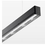
Light band with LED, rated life of the LED L80/B50 > 50000 h, colour rendering index CRI > 80, reflector with double asymmetrical light distribution pattern, lens optics made of PMMA, luminaire insert sheet steel, powder-coated, black
