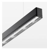
Light band with LED, rated life of the LED L80/B50 > 50000 h, colour rendering index CRI > 80, reflector with double asymmetrical light distribution pattern, lens optics made of PMMA, luminaire insert sheet steel, powder-coated, black
