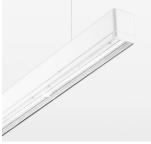
Light band with LED, rated life of the LED L80/B50 > 50000 h, colour rendering index CRI > 80, reflector with homogeneous light distribution pattern, lens optics made of PMMA, luminaire insert sheet steel, powder-coated, white
