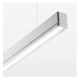
Light band with LED, rated life of the LED L80/B50 > 50000 h, colour rendering index CRI > 80, reflector with homogeneous light distribution pattern, lens optics made of PMMA, luminaire insert sheet steel, powder-coated, silver
