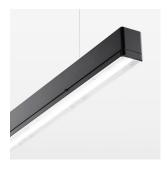
Light band with LED, rated life of the LED L80/B50 > 50000 h, colour rendering index CRI > 80, reflector with homogeneous light distribution pattern, lens optics made of PMMA, luminaire insert sheet steel, powder-coated, black
