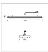
Lay in luminaire with LED, rated life of the LED L80/B50 > 50000 h, colour rendering index CRI > 80, chromaticity tolerance 3 SDCM (initial), wide, homogeneous light distribution pattern, TIR-lens made of PMMA, luminaire housing sheet steel, powder-coated, matt white
