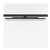
Surface-mounted luminaire with LED, rated life of the LED L80/B50 > 50000 h, colour rendering index CRI > 80, chromaticity tolerance 3 SDCM (initial), extra wide, homogeneous light distribution pattern, TIR-lens made of PMMA, power selection via DIP switch, 8 possible levels: 38 W (5530 lm), 42 W (6130 lm), 47 W (6700 lm), 52 W (7280 lm), 57 W (7850 lm , preset), 62W (8390 lm), 67 W (8950 lm), 72 W (9490 lm), rotation angle 330°, luminaire housing sheet steel, powder-coated, matt black,
