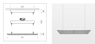
Suspended luminaire with LED, rated life of the LED L80/B50 > 50000 h, colour rendering index CRI > 80, chromaticity tolerance 3 SDCM (initial), double asymmetrical light distribution pattern, lens made of PMMA, luminaire housing sheet steel, powder-coated, matt white, power supply via suspension cables
