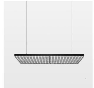
Suspended luminaire with LED, rated life of the LED L80/B50 > 50000 h, colour rendering index CRI > 80, chromaticity tolerance 3 SDCM (initial), wide, homogeneous light distribution pattern, TIR-lens made of PMMA, luminaire housing sheet steel, powder-coated, matt black, power supply via suspension cables
