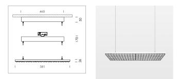
Suspended luminaire with LED, rated life of the LED L80/B50 > 50000 h, colour rendering index CRI > 80, chromaticity tolerance 3 SDCM (initial), wide, homogeneous light distribution pattern, TIR-lens made of PMMA, luminaire housing sheet steel, powder-coated, matt white, power supply via suspension cables
