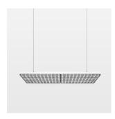
Suspended luminaire with LED, rated life of the LED L80/B50 > 50000 h, colour rendering index CRI > 80, chromaticity tolerance 3 SDCM (initial), wide, homogeneous light distribution pattern, TIR-lens made of PMMA, luminaire housing sheet steel, powder-coated, matt white, power supply via suspension cables
