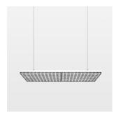
Suspended luminaire with LED, rated life of the LED L80/B50 > 50000 h, colour rendering index CRI > 80, chromaticity tolerance 3 SDCM (initial), wide, homogeneous light distribution pattern, TIR-lens made of PMMA, luminaire housing sheet steel, powder-coated, matt white, power supply via suspension cables
