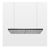
Suspended luminaire with LED, rated life of the LED L80/B50 > 50000 h, colour rendering index CRI > 80, chromaticity tolerance 3 SDCM (initial), extra wide, homogeneous light distribution pattern, TIR-lens made of PMMA, luminaire housing sheet steel, powder-coated, matt black, power supply via suspension cables
