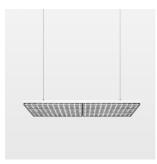
Suspended luminaire with LED, rated life of the LED L80/B50 > 50000 h, colour rendering index CRI > 80, chromaticity tolerance 3 SDCM (initial), extra wide, homogeneous light distribution pattern, TIR-lens made of PMMA, luminaire housing sheet steel, powder-coated, matt white, power supply via suspension cables
