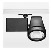
Surface-mounted luminaire with LED, rated life of the LED L80/B10 > 50000 h, chromaticity tolerance 2 SDCM (initial), reflector with circular light distribution pattern, reflector pure aluminium 99,99% in MIRO-Silver®, rotation angle 350°, swivel angle 210°, luminaire housing die-cast aluminium, powder-coated, stratoblack
