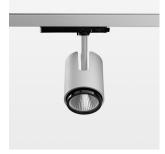
Surface-mounted luminaire with LED, rated life of the LED L80/B10 > 50000 h, chromaticity tolerance 2 SDCM (initial), , reflector with circular light distribution pattern, reflector pure aluminium 99,99% in MIRO-Silver®, segmented and faceted, exchangeable reflector unit in high-sheen black plastic, with glass cover, luminaire head die-cast aluminium, powder-coated, rotation angle 330°, swivel angle +/-90°, luminaire head/retention arm die-cast aluminium, stratosilver
