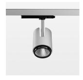
Surface-mounted luminaire with LED, rated life of the LED L80/B10 > 50000 h, chromaticity tolerance 3 SDCM (initial), , reflector with circular light distribution pattern, reflector pure aluminium 99,99% in MIRO-Silver®, segmented and faceted, exchangeable reflector unit in high-sheen black plastic, with glass cover, luminaire head die-cast aluminium, powder-coated, rotation angle 330°, swivel angle +/-90°, luminaire head/retention arm die-cast aluminium, stratosilver
