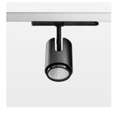
Surface-mounted luminaire with LED, rated life of the LED L80/B10 > 50000 h, chromaticity tolerance 3 SDCM (initial), , reflector with circular light distribution pattern, reflector pure aluminium 99,99% in MIRO-Silver®, segmented and faceted, exchangeable reflector unit in high-sheen black plastic, with glass cover, luminaire head die-cast aluminium, powder-coated, rotation angle 330°, swivel angle +90°/-90°, luminaire head/retention arm die-cast aluminium, stratoblack
