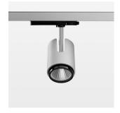
Surface-mounted luminaire with LED, rated life of the LED L80/B10 > 50000 h, chromaticity tolerance 2 SDCM (initial), , reflector with circular light distribution pattern, reflector pure aluminium 99,99% in MIRO-Silver®, segmented and faceted, exchangeable reflector unit in high-sheen black plastic, with glass cover, luminaire head die-cast aluminium, powder-coated, rotation angle 330°, swivel angle +90°/-90°, luminaire head/retention arm die-cast aluminium, stratosilver
