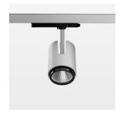
Surface-mounted luminaire with LED, rated life of the LED L80/B10 > 50000 h, chromaticity tolerance 3 SDCM (initial), , reflector with circular light distribution pattern, reflector pure aluminium 99,99% in MIRO-Silver®, segmented and faceted, exchangeable reflector unit in high-sheen black plastic, with glass cover, luminaire head die-cast aluminium, powder-coated, rotation angle 330°, swivel angle +90°/-90°, luminaire head/retention arm die-cast aluminium, stratosilver
