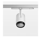
Surface-mounted luminaire with LED, rated life of the LED L80/B10 > 50000 h, chromaticity tolerance 2 SDCM (initial), , reflector with circular light distribution pattern, reflector pure aluminium 99,99% in MIRO-Silver®, segmented and faceted, exchangeable reflector unit in high-sheen black plastic, with glass cover, luminaire head die-cast aluminium, powder-coated, rotation angle 330°, swivel angle +90°/-90°, luminaire head/retention arm die-cast aluminium, stratowhite
