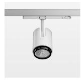
Surface-mounted luminaire with LED, rated life of the LED L80/B10 > 50000 h, chromaticity tolerance 3 SDCM (initial), , reflector with circular light distribution pattern, reflector pure aluminium 99,99% in MIRO-Silver®, segmented and faceted, exchangeable reflector unit in high-sheen black plastic, with glass cover, luminaire head die-cast aluminium, powder-coated, rotation angle 330°, swivel angle +90°/-90°, luminaire head/retention arm die-cast aluminium, special colour
