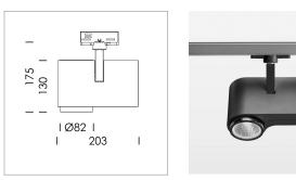
Surface-mounted luminaire with LED, rated life of the LED L80/B10 > 50000 h, colour rendering index CRI > 96, chromaticity tolerance 3 SDCM (initial), reflector with circular light distribution pattern, reflector pure aluminium 99,99% in MIRO-Silver®, segmented and faceted, exchangeable reflector unit in high-sheen black plastic, with glass cover, rotation angle 330°, swivel angle 90°, luminaire housing die-cast aluminium, powder-coated, stratoblack
