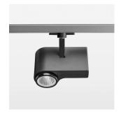
Surface-mounted luminaire with LED, rated life of the LED L80/B10 > 50000 h, chromaticity tolerance 3 SDCM (initial), reflector with circular light distribution pattern, reflector pure aluminium 99,99% in MIRO-Silver®, segmented and faceted, exchangeable reflector unit in high-sheen black plastic, with glass cover, rotation angle 330°, swivel angle 90°, luminaire housing diecast aluminium, powder-coated, stratoblack
