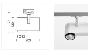
Surface-mounted luminaire with LED, rated life of the LED L80/B10 > 50000 h, chromaticity tolerance 3 SDCM (initial), reflector with circular light distribution pattern, reflector pure aluminium 99,99% in MIRO-Silver®, segmented and faceted, exchangeable reflector unit in high-sheen black plastic, with glass cover, rotation angle 330°, swivel angle 90°, luminaire housing diecast aluminium, powder-coated, stratowhite
