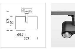
Surface-mounted luminaire with LED, rated life of the LED L80/B10 > 50000 h, colour rendering index CRI > 90, chromaticity tolerance 2 SDCM (initial), reflector with circular light distribution pattern, reflector pure aluminium 99,99% in MIRO-Silver®, segmented and faceted, exchangeable reflector unit in high-sheen black plastic, with glass cover, rotation angle 330°, swivel angle 90°, luminaire housing die-cast aluminium, powder-coated, stratoblack
