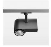
Surface-mounted luminaire with LED, rated life of the LED L80/B10 > 50000 h, colour rendering index CRI > 96, chromaticity tolerance 3 SDCM (initial), reflector with circular light distribution pattern, reflector pure aluminium 99,99% in MIRO-Silver®, segmented and faceted, exchangeable reflector unit in high-sheen black plastic, with glass cover, rotation angle 330°, swivel angle 90°, luminaire housing die-cast aluminium, powder-coated, stratoblack
