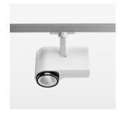
Surface-mounted luminaire with LED, rated life of the LED L80/B10 > 50000 h, colour rendering index CRI > 80, chromaticity tolerance 2 SDCM (initial), reflector with circular light distribution pattern, reflector pure aluminium 99,99% in MIRO-Silver®, segmented and faceted, exchangeable reflector unit in high-sheen black plastic, with glass cover, rotation angle 330°, swivel angle 90°, luminaire housing die-cast aluminium, powder-coated, stratowhite
