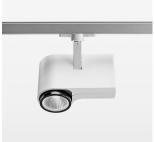
Surface-mounted luminaire with LED, rated life of the LED L80/B10 > 50000 h, colour rendering index CRI > 96, chromaticity tolerance 2 SDCM (initial), reflector with circular light distribution pattern, reflector pure aluminium 99,99% in MIRO-Silver®, segmented and faceted, exchangeable reflector unit in high-sheen black plastic, with glass cover, rotation angle 330°, swivel angle 90°, luminaire housing die-cast aluminium, powder-coated, stratowhite
