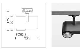
Surface-mounted luminaire with LED, rated life of the LED L80/B10 > 50000 h, colour rendering index CRI > 96, chromaticity tolerance 2 SDCM (initial), reflector with circular light distribution pattern, reflector pure aluminium 99,99% in MIRO-Silver®, segmented and faceted, exchangeable reflector unit in high-sheen black plastic, with glass cover, rotation angle 330°, swivel angle 90°, luminaire housing die-cast aluminium, powder-coated, stratoblack
