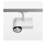
Surface-mounted luminaire with LED, rated life of the LED L80/B10 > 50000 h, colour rendering index CRI > 80, chromaticity tolerance 2 SDCM (initial), reflector with circular light distribution pattern, reflector pure aluminium 99,99% in MIRO-Silver®, segmented and faceted, exchangeable reflector unit in high-sheen black plastic, with glass cover, rotation angle 330°, swivel angle 90°, luminaire housing die-cast aluminium, powder-coated, stratowhite
