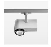
Surface-mounted luminaire with LED, rated life of the LED L80/B10 > 50000 h, chromaticity tolerance 2 SDCM (initial), LED hybrid technology, 3D silicone lens to reduce the proportion of scattered light, reflector with oval light distribution pattern, reflector pure aluminium 99,99% in MIRO-Silver®, segmented, exchangeable reflector unit in high-sheen black plastic, with glass cover, rotation angle 330°, swivel angle 90°, luminaire housing die-cast aluminium, powder-coated, stratosilver
