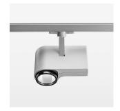
Surface-mounted luminaire with LED, rated life of the LED L80/B10 > 50000 h, chromaticity tolerance 2 SDCM (initial), LED hybrid technology, 3D silicone lens to reduce the proportion of scattered light, reflector with oval light distribution pattern, reflector pure aluminium 99,99% in MIRO-Silver®, segmented, exchangeable reflector unit in high-sheen black plastic, with glass cover, rotation angle 330°, swivel angle 90°, luminaire housing die-cast aluminium, powder-coated, stratosilver
