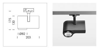
Surface-mounted luminaire with LED, rated life of the LED L80/B10 > 50000 h, chromaticity tolerance 3 SDCM (initial), LED hybrid technology, 3D silicone lens to reduce the proportion of scattered light, reflector with oval light distribution pattern, reflector pure aluminium 99,99% in MIRO-Silver®, segmented, exchangeable reflector unit in high-sheen black plastic, with glass cover, rotation angle 330°, swivel angle 90°, luminaire housing die-cast aluminium, powder-coated, stratoblack
