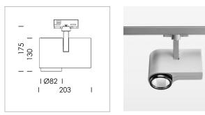
Surface-mounted luminaire with LED, rated life of the LED L80/B10 > 50000 h, chromaticity tolerance 2 SDCM (initial), LED hybrid technology, 3D silicone lens to reduce the proportion of scattered light, reflector with oval light distribution pattern, reflector pure aluminium 99,99% in MIRO-Silver®, segmented, exchangeable reflector unit in high-sheen black plastic, with glass cover, rotation angle 330°, swivel angle 90°, luminaire housing die-cast aluminium, powder-coated, stratosilver
