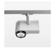
Surface-mounted luminaire with LED, rated life of the LED L80/B10 > 50000 h, chromaticity tolerance 3 SDCM (initial), LED hybrid technology, 3D silicone lens to reduce the proportion of scattered light, reflector with oval light distribution pattern, reflector pure aluminium 99,99% in MIRO-Silver®, segmented, exchangeable reflector unit in high-sheen black plastic, with glass cover, rotation angle 330°, swivel angle 90°, luminaire housing die-cast aluminium, powder-coated, stratosilver
