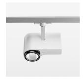
Surface-mounted luminaire with LED, rated life of the LED L80/B10 > 50000 h, chromaticity tolerance 2 SDCM (initial), LED hybrid technology, 3D silicone lens to reduce the proportion of scattered light, reflector with oval light distribution pattern, reflector pure aluminium 99,99% in MIRO-Silver®, segmented, exchangeable reflector unit in high-sheen black plastic, with glass cover, rotation angle 330°, swivel angle 90°, luminaire housing die-cast aluminium, powder-coated, stratowhite
