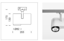
Surface-mounted luminaire with LED, rated life of the LED L80/B10 > 50000 h, chromaticity tolerance 3 SDCM (initial), LED hybrid technology, 3D silicone lens to reduce the proportion of scattered light, reflector with oval light distribution pattern, reflector pure aluminium 99,99% in MIRO-Silver®, segmented, exchangeable reflector unit in high-sheen black plastic, with glass cover, rotation angle 330°, swivel angle 90°, luminaire housing die-cast aluminium, powder-coated, stratowhite
