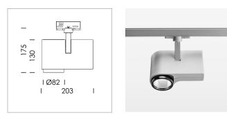
Surface-mounted luminaire with LED, rated life of the LED L80/B10 > 50000 h, chromaticity tolerance 3 SDCM (initial), LED hybrid technology, 3D silicone lens to reduce the proportion of scattered light, reflector with oval light distribution pattern, reflector pure aluminium 99,99% in MIRO-Silver®, segmented, exchangeable reflector unit in high-sheen black plastic, with glass cover, rotation angle 330°, swivel angle 90°, luminaire housing die-cast aluminium, powder-coated, stratosilver
