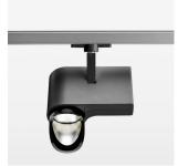
Surface-mounted luminaire with LED, rated life of the LED L80/B10 > 50000 h, chromaticity tolerance 3 SDCM (initial), reflector with asymmetrical light distribution pattern, primary reflector and kick reflector 99% pure aluminium in MIRO-Silver®, attachment with kick reflector to the ceiling approach of the light cone, exchangeable reflector unit in high-sheen black plastic, with glass cover, rotation angle 330°, swivel angle 90°, luminaire housing die-cast aluminium, powder-coated, stratoblack
