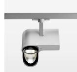
Surface-mounted luminaire with LED, rated life of the LED L80/B10 > 50000 h, chromaticity tolerance 3 SDCM (initial), reflector with asymmetrical light distribution pattern, primary reflector and kick reflector 99% pure aluminium in MIRO-Silver®, attachment with kick reflector to the ceiling approach of the light cone, exchangeable reflector unit in high-sheen black plastic, with glass cover, rotation angle 330°, swivel angle 90°, luminaire housing die-cast aluminium, powder-coated, stratosilver
