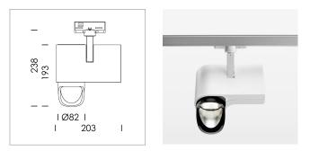
Surface-mounted luminaire with LED, rated life of the LED L80/B10 > 50000 h, chromaticity tolerance 3 SDCM (initial), reflector with asymmetrical light distribution pattern, primary reflector and kick reflector 99% pure aluminium in MIRO-Silver®, attachment with kick reflector to the ceiling approach of the light cone, exchangeable reflector unit in high-sheen black plastic, with glass cover, rotation angle 330°, swivel angle 90°, luminaire housing die-cast aluminium, powder-coated, stratowhite
