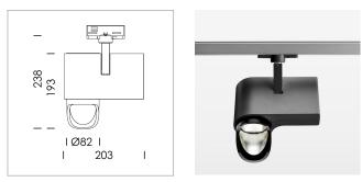
Surface-mounted luminaire with LED, rated life of the LED L80/B10 > 50000 h, chromaticity tolerance 2 SDCM (initial), reflector with asymmetrical light distribution pattern, primary reflector and kick reflector 99% pure aluminium in MIRO-Silver®, attachment with kick reflector to the ceiling approach of the light cone, exchangeable reflector unit in high-sheen black plastic, with glass cover, rotation angle 330°, swivel angle 90°, luminaire housing die-cast aluminium, powder-coated, stratoblack
