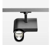
Surface-mounted luminaire with LED, rated life of the LED L80/B10 > 50000 h, chromaticity tolerance 3 SDCM (initial), reflector with asymmetrical light distribution pattern, primary reflector and kick reflector 99% pure aluminium in MIRO-Silver®, attachment with kick reflector to the ceiling approach of the light cone, exchangeable reflector unit in high-sheen black plastic, with glass cover, rotation angle 330°, swivel angle 90°, luminaire housing die-cast aluminium, powder-coated, stratoblack
